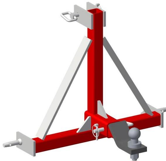
This trailer towbar hitch adapter for tractors is simple to make and quick to hook up to the three point linkage of the tractor to move a trailer around the farm.
